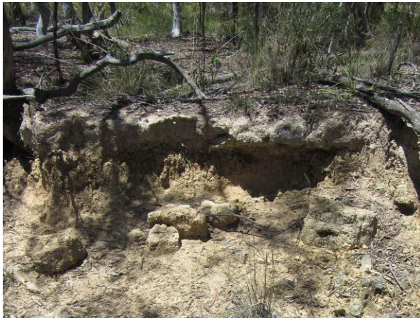
Fig. 9. An example of erosion in an exposed sodic texture contrast soil. The yellow-coloured clay-rich B horizon is eroded by undercutting or ‘caving’, ultimately allowing the more stable A horizon to simply fall away (mass wasting). Photo: D Tongway.
